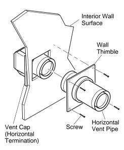
Figure 25 - Connecting Vent Cap with Horizontal Vent Pipe
